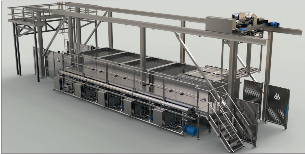
▲ Photo 3: Automatic cook processing system: COOKLINE.
