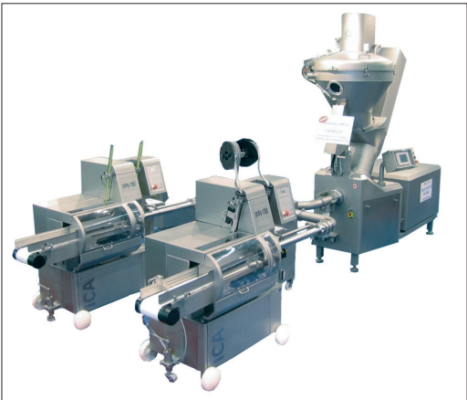
▲ Photo 4: Dual Stuffing / Clipping System: TWINVAC + TWINCLIP.
