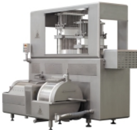
The Movistick 4500 CR bone in/boneless spray injector.
